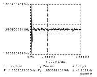
FIGURE 13. Frequency Jump Lock Time
