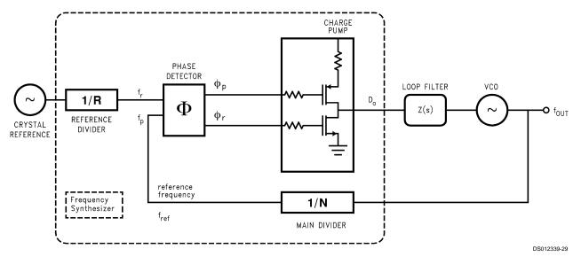
FIGURE 1. Basic Charge Pump Phase Locked Loop
