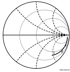
Marker 1 = 500 MHz, Real = 69, Imag. = -330 Marker 2 = 900 MHz, Real = 36, Imag. = -193 Marker 3 = 1 GHz, Real = 35, Imag. = -172 Marker 4 = 1,500 MHz, Real = 30, Imag. = -106
