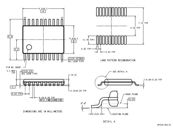
**NS Package Number MTC20** 20-Lead (0.173" Wide) Thin Shrink Small Outline Package (TM) Order Number LMX2315TM, LMX2320TM or LMX2325TM For Tape and Reel Order Number LMX2315TMX, LMX2320TMX or LMX2325TMX (2500 Units per Reel)
