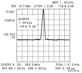
FIGURE 7. PLL Phase Noise @ 1 kHz Offset
