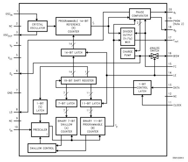
Note 1: The prescalar for the LMX2315 and LMX2320 is either 64/65 or 128/129, while the prescalar for the LMX2325 is 32/33 or 64/65.
