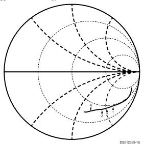
1 = 1.5 GHz, Real = 48, Im = -128 2 = 1.8 GHz, Real = 44, Im = -102 3 = 2.0 GHz, Real = 42, Im = -90 4 = 2.5 GHz, Real = 36, Im = -72
