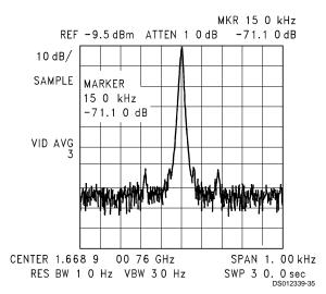
FIGURE 11. PLL Phase Noise @ 150 Hz Offset
