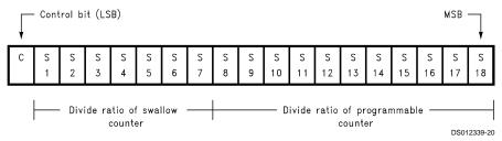
Note: S8 to S18: Programmable counter divide ratio control bits (3 to 2047)
