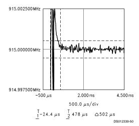
FIGURE 8. Frequency Jump Lock Time
