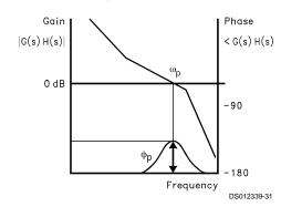
FIGURE 3. Open Loop Transfer Function
